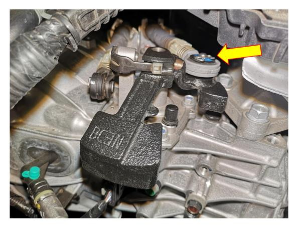
8. There is a C-clip that holds the up/down shifter mechanism in place.
