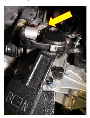
10. To remove the pin, you will need a punch/suitable tool that is around 4mm diameter. Place this into the hole in the OEM shifter and hit the punch/suitable tool with a hammer/mallet until the pin is no longer impairing the centre bore so the OEM shifter can be lifted off vertically. We recommend not to hit the pin the full way through the shifter. Again, placing a magnet behind the shifter can be beneficial in case you hit the pin out of the OEM shifter.
